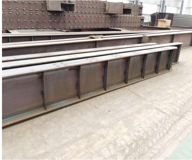
H-shaped structural stiffener welding
