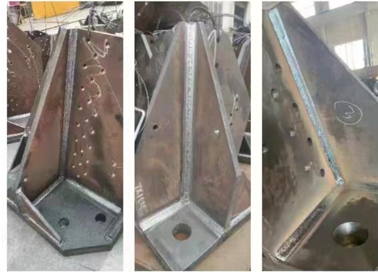
Tower corner welding
